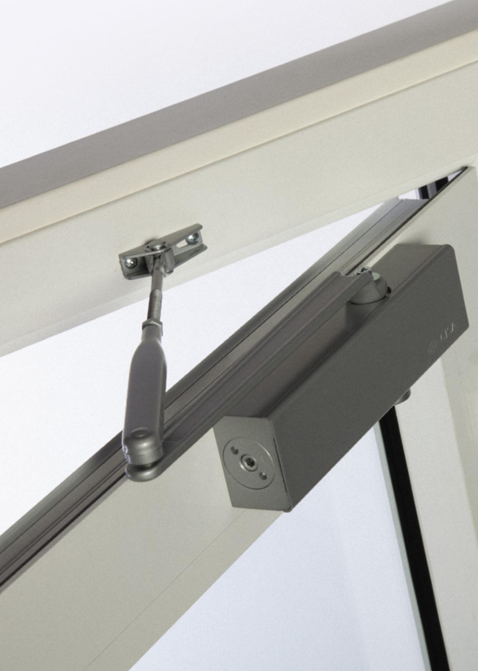
Adjusting strength and maximum door dimensions. The closer body remains in a fixed position. The closing force of the door is adjusted by changing the position of the arm support and turning the screw on the side.
