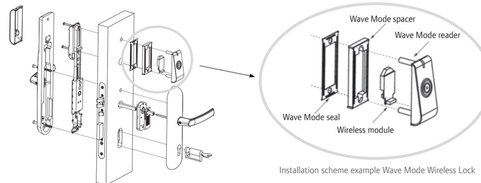
Installation scheme example Wave Mode Wireless Lock
